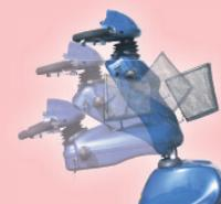
Angle adjustable steering column, stepless and operable from the steering column.
