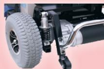
Equipped with independent suspension on the front and rear. Also easily adjustable rear suspension.
